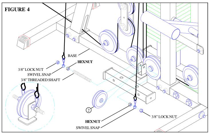
• Assemble the two previously removed 3/8" HEX NUTS, two previously removed SWIVEL SNAPS, one 3-1/2" PULLEY (2), and two previously removed 3/8" LOCK NUTS to the previously removed 3/8" THREADED SHAFT as shown in FIGURE 4.
